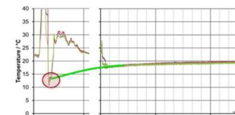
The data above show the temperature profiles within the mould and inside the ampoule. The BFS process with cooling shows that temperature can be controlled within a range that is acceptable for proteins.
