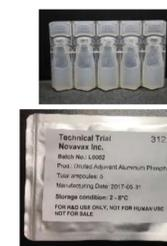
Limited water loss even if BFS containers were not stored in gas / moisture barrier secondary packaging
